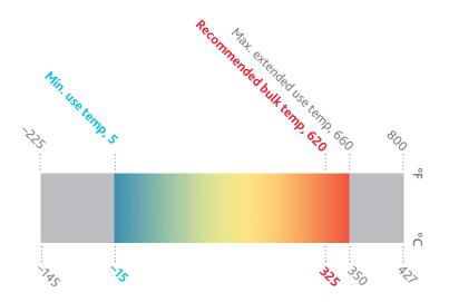
Eastman Marlotherm® SH heat transfer fluid is a synthetic heat transfer fluid that offers outstanding performance during both low-temperature start-up and high-temperature operation. It performs over the entire temperature range without being kept under pressure. When operating in a well-maintained heat transfer system, Marlotherm SH provides reliable, consistent performance over long periods of time.
